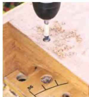
STEP 21. Drill a 13mm hole into the rear face of each end piece; this creates clearance
